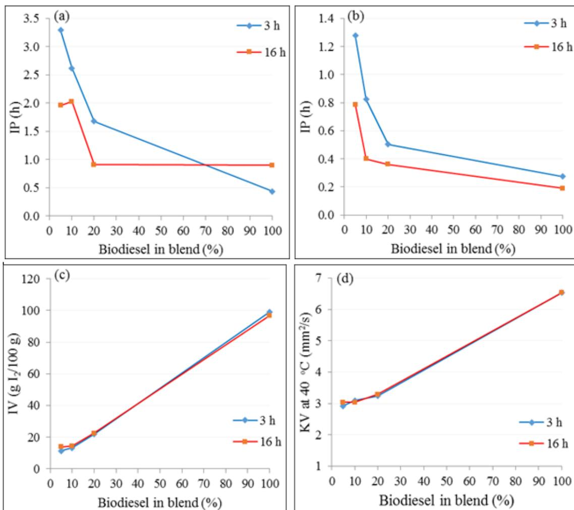
**Fig. 2: Results of oxidation stability after strip corrosion test at 115°C: Rancimat test (a), PetroOXY test (b), Iodine value (c), and kinematic viscosity at 40°C (d)**
