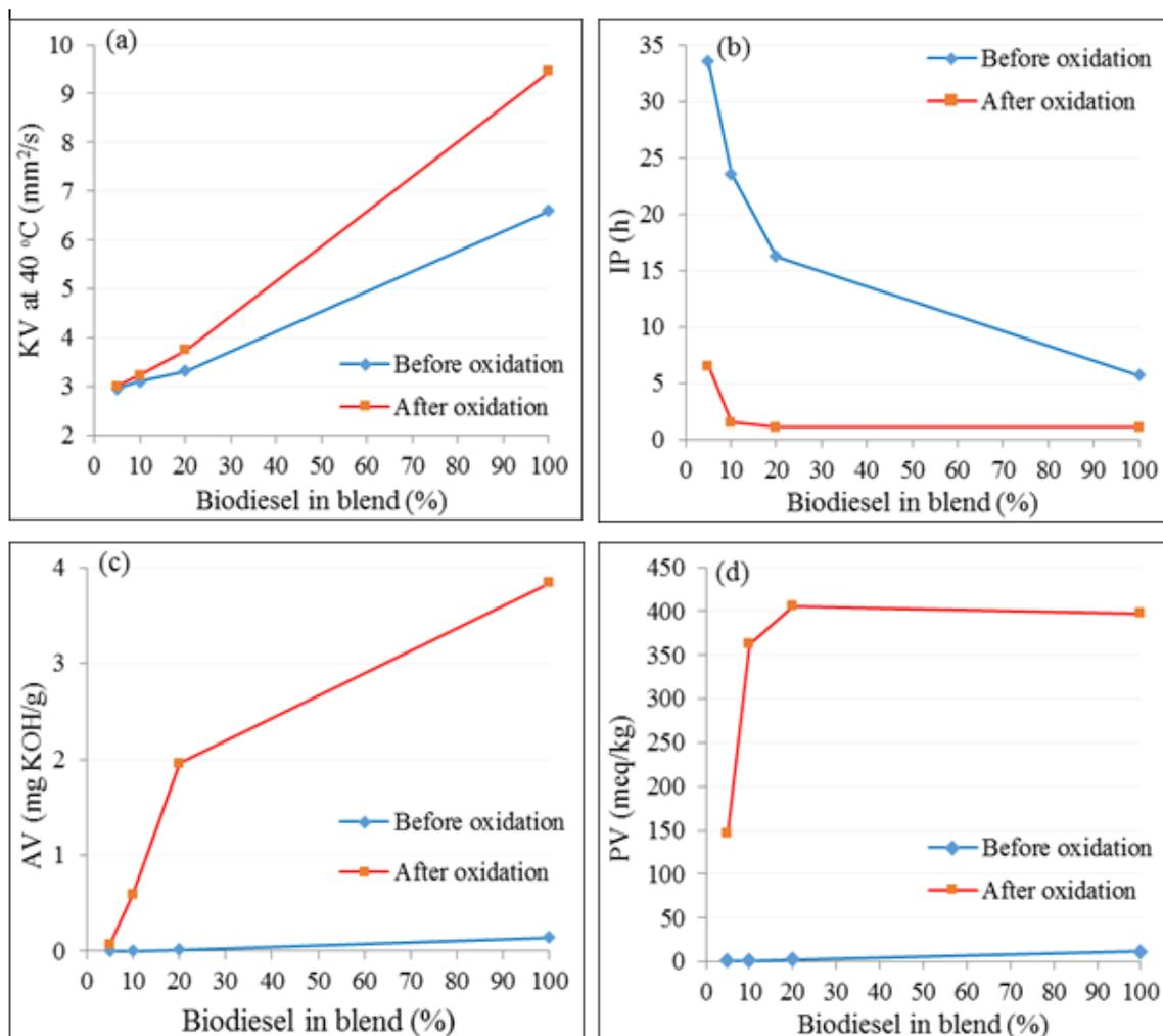
Fig. 3: Results of kinematic viscosity at 40°C (a), Rancimat test (b), acid value (c), and peroxide test (d) before and after the oxidation test at 115°C for 16 hrs. under bubbling oxygen
